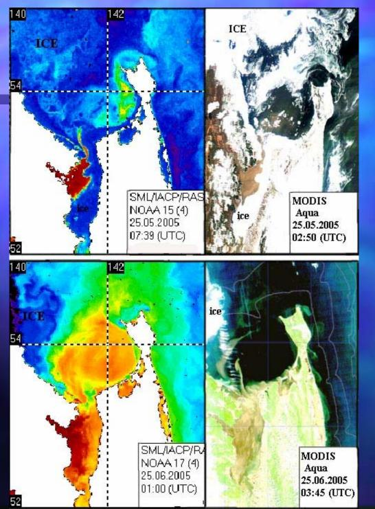
Satellite – acquired data can provide information on the distribution of the Amur River water and sediments on the continental shelf of the Sea of Okhotsk. This figure shows the IR **AVHHR images (left panel) and MODIS true color (bands 1-4-3)** images (right panel). During spring-summer flood the jet –like outflow from the Liman forms the Amur River plume and associated frontal structure in the Sakhalin Bay.
